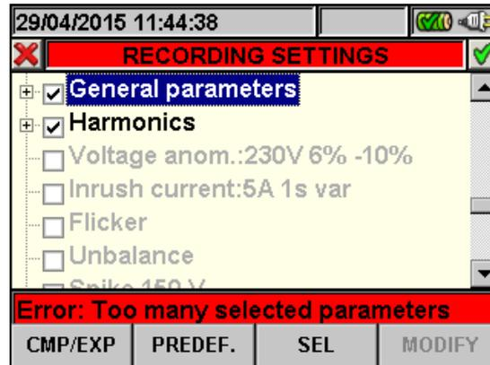
Fig. 68: General Parameters section: too many selected parameters
