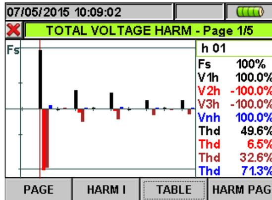
Fig. 33: Harmonic analysis of voltages in percentage value for 4-wire systems
