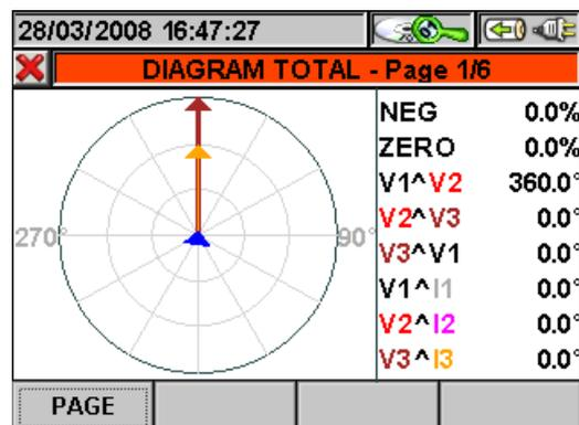
Fig. 118: Total vector diagram in three-phase 4-wire system
