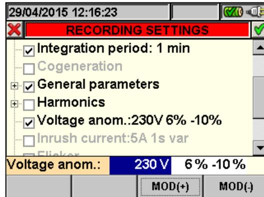
Fig. 75: Voltage Anomalies screen - setting control parameters
