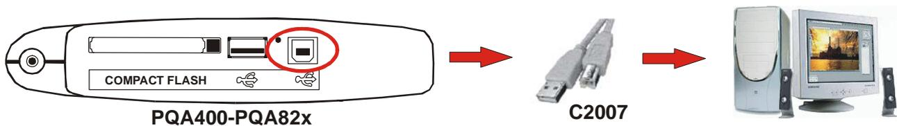
Fig. 128: Connection of meter to PC
