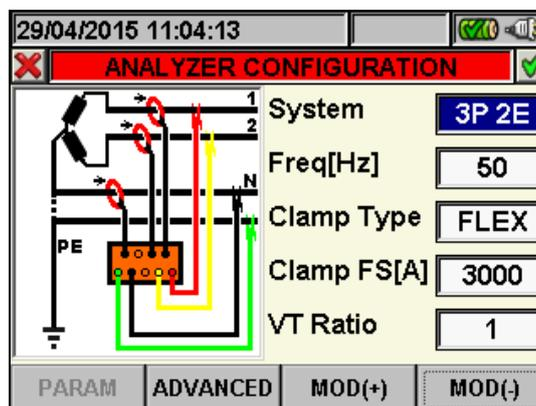
Fig. 55: Analyzer Configuration screen for 2-phase system 3-wire 3P 2E – ENG\_UK type
