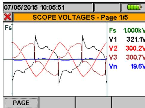
Fig. 28: Voltage waveforms screen for 4-wire systems
