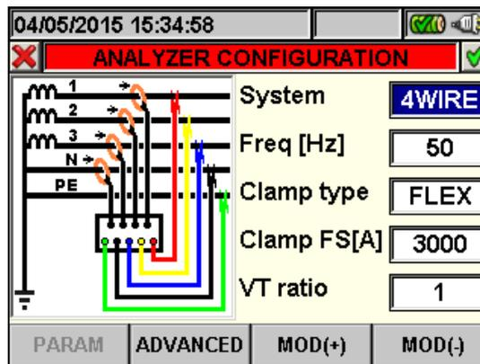
Fig. 45: Analyzer configuration screen for 4-wire system – ENG\_UK type
