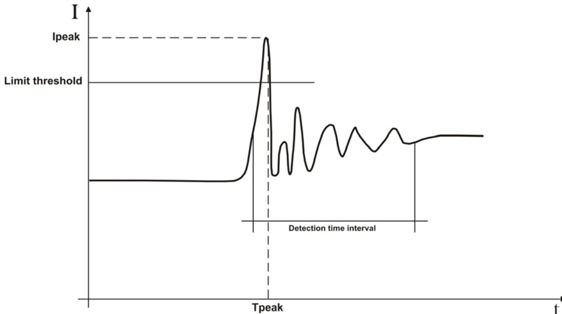
Fig. 149: Parameters of oscillating inrush current event
