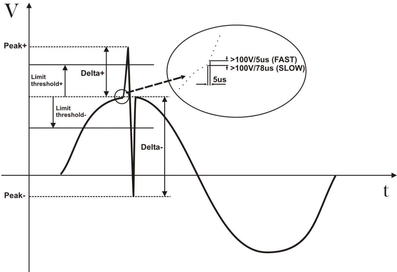
Fig. 151: Typical voltage spikes at 50Hz frequency
