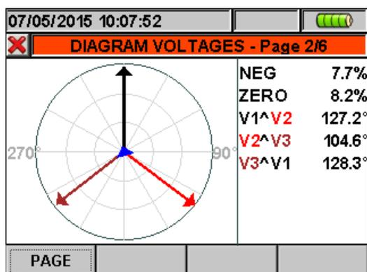
Fig. 40: Vectorial voltage diagram for 4-wire system
