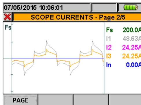
Fig. 29: Current waveforms screen for 4-wire systems
