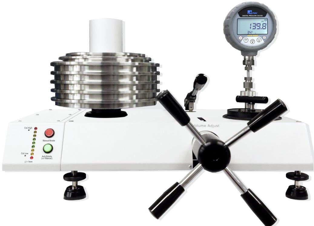
**Dead-Weight Tester** is used as a generator of an accurately known pressure. It measures pressure as force per unit area. Therefore, Dead-Weight Tester is the most accurate pressure calibrator.
