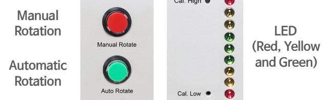
In order to rotate piston, two methods are available. The first one is to press the red button on the front panel of PDPG-HI. The piston can be rotated only when you want to rotate. Second method is to press the green button. When the piston is located in a suitable operation position, the piston rotates automatically. The operation interval covers  $\pm 3$  mm from reference float line. If out of range, piston stops automatically.
